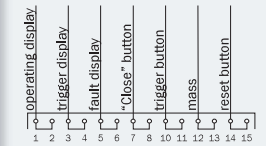
Connection allocation smoke and heat ventilation button 6
